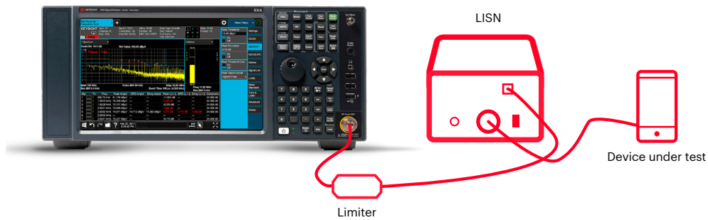
Figure 4. A transient limiter + LISN are used during conducted emissions testing
