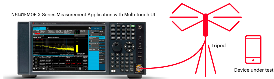
Figure 3. A signal analyzer with an EMC application and a calibrated EMI antenna are used during radiated emissions testing
