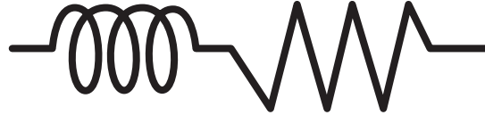
Figure 1. Equivalent circuit of a ferrite bead
