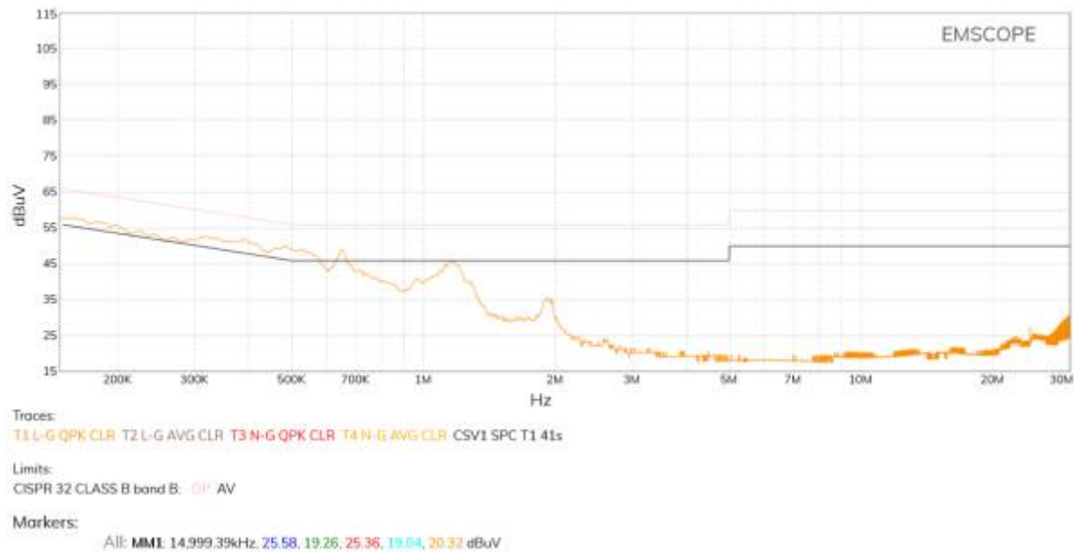
Figure 14. QPK Line emissions at a specific time slice where the cavity magnetron is on. Equipment with the designed filter.
