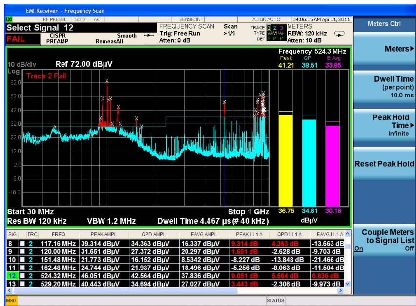
Figure 3. Signal list measurement results automatically collected by the MXE
