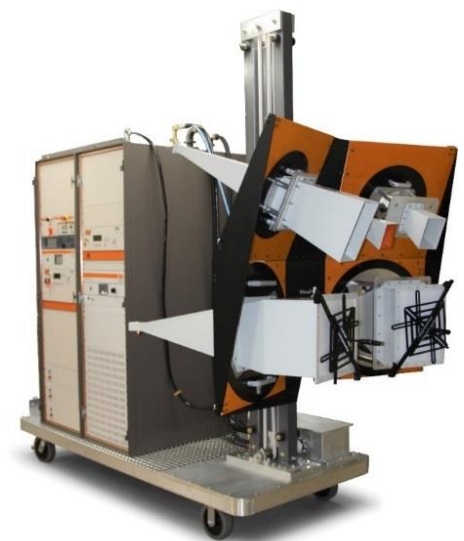
Figure 14: Mobile Radiated Immunity Test System
